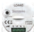
ZM-LD440 Dimmer for LED lamp Power: 440W 230V 50/60 Hz Installed in the mounting box behind the push button. Dimensions: 56 x 22 mm Units: 1
