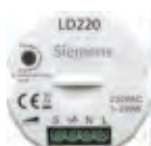
ZM-LD220 Dimmer for LED lamp Power: 200W 230 V 50/60 Hz Installed in the mounting box behind the push button. Dimensions: 56 x 22 mm Units: 1
